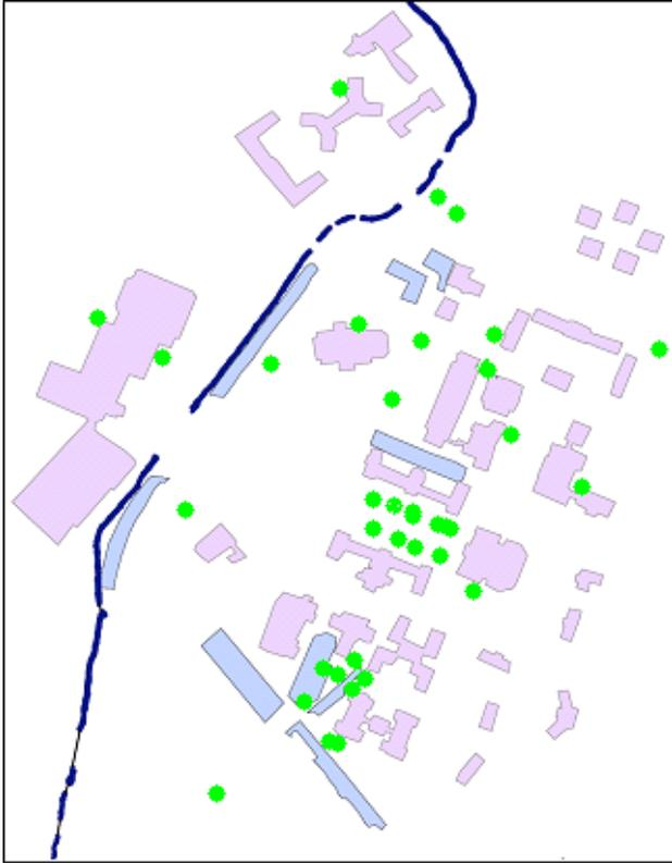
**Figure 3-4** Locations where rain gardens could be aligned with Bucknell's storm drainage system.
