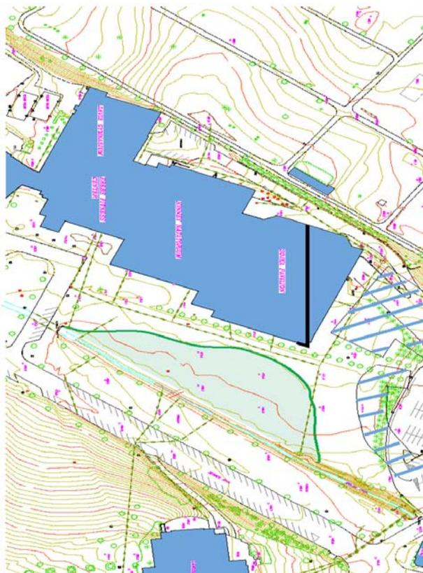
**Figure 3-9** Reach 2a showing the proposed Bucknell Inn (cross-hatched) and proposed wetland (green area on Sojka Lawn) for stormwater retention and low-flow augmentation of Miller Run.
