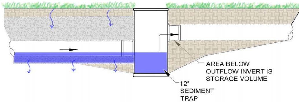
**Figure 3-5** Cross-section diagram of an infiltration trench. Water would flow along the deep pipe, which is perforated to allow infiltration, and be stored in the trap to allow sediment deposition and further infiltration. Water would only reach the shallow pipe when enough runoff entered the system to elevate the level in the trap.
