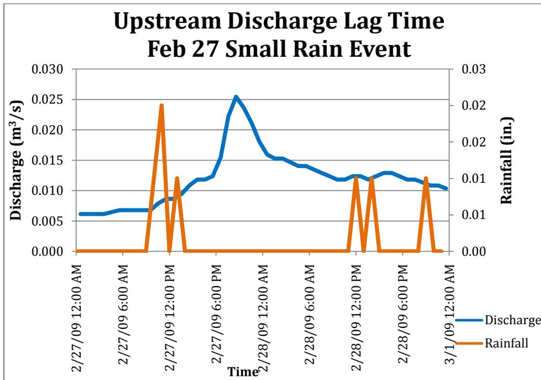
Figure 2-14. Lag between Rainfall and Upstream Discharge for a Small Feb 27 Rain Event
