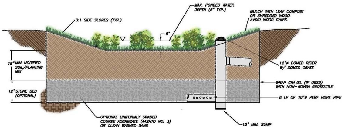
**Figure 3-2** Cross-section through a rain garden, showing depression to collect storm water and the overflow pipe connected to underground sump and perforated pipe connected to storm water drainage system. On this diagram, water would enter the overflow pipe once it reaches 6 inches deep.
